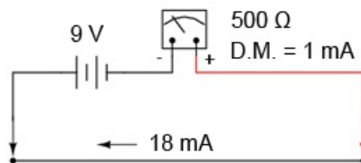
Figure 282: ohmmetru analogic
